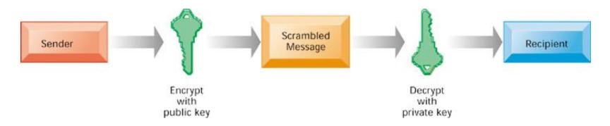
A public key encryption system can be viewed as a series of public and private keys that lock data when they are transmitted and unlock the data when they are received. The sender locates the recipient's public key in a directory and uses it to encrypt a message. The message is sent in encrypted form over the Internet or a private network. When the encrypted message arrives, the recipient uses his or her private key to decrypt the data and read the message.
