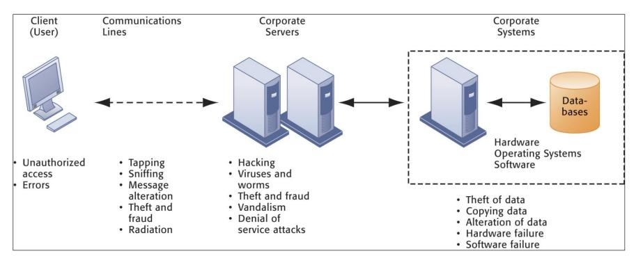
The architecture of a Web-based application typically includes a Web client, a server, and corporate information systems linked to databases. Each of these components presents security challenges and vulnerabilities. Floods, fires, power failures, and other electrical problems can cause disruptions at any point in the network.
